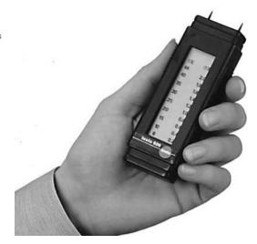
Part no. 0560 6061 Technical data Electrodes: integrated, exchangeable, 8 mm los Applications: Wood, wood products, veneer,
